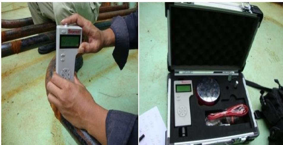
Gambar 3.6 Digital Hardness Tester
