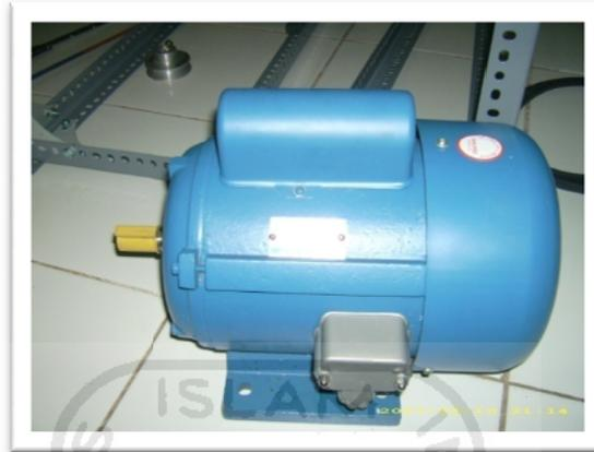
**Gambar 3.8** Motor AC 1 phase  $\frac{3}{4}$ HP 1400rpm
