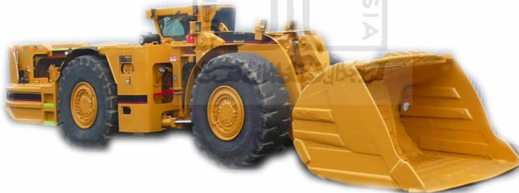
Gambar 4.2 Load Haul Dump
