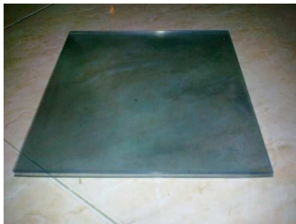
Gambar 3.5 Lembaran plastik PET ( polyethylene terephthalate )
