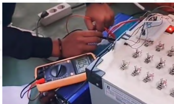
Gambar 3.7 Proses Kalibrasi Sensor PZEM-004T-100A Split Core
