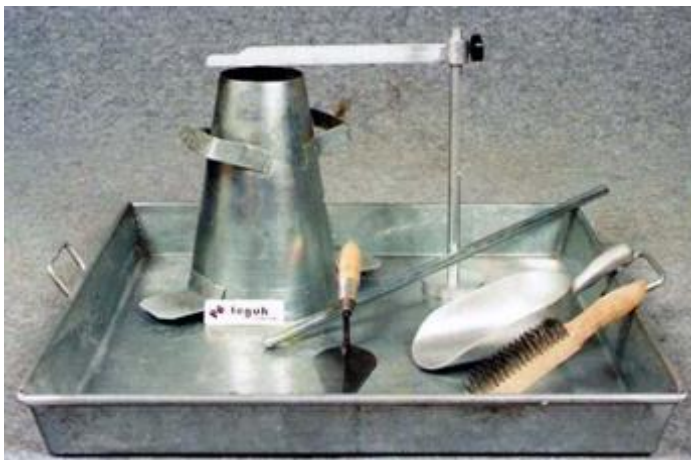
Gambar 4.9 Slump test set
