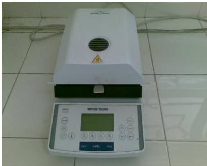
Alat uji kadar air ( Moisture balance )
