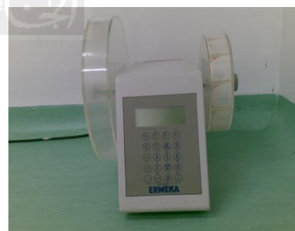
Alat uji kerapuhan tablet ( Friability tester )
