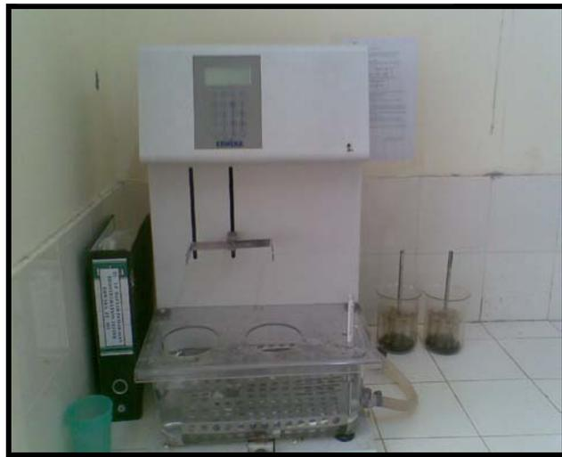
**Gambar 12.** Alat *Disintegration Tester*
