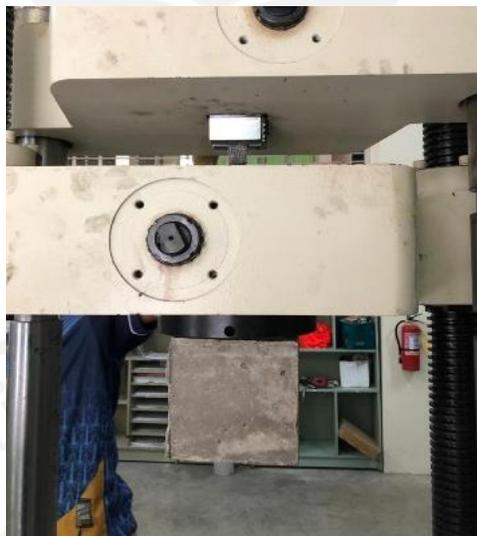
**Gambar 5.28 Benda Uji *Pull Out***
