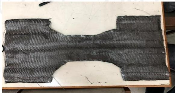
**Gambar 5.14 Benda Uji Carbon Fiber Trial IV Sebelum Digulung**
