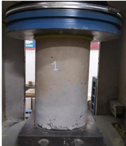
**Gambar 5.27 Pengujian *Trial Mix Design* Silinder Beton**
