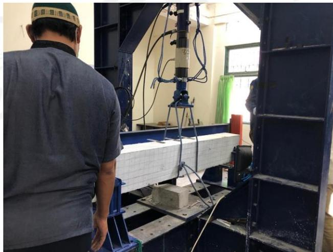
GAMBAR 38 PENGUJIAN BERAT BALOK BETON
