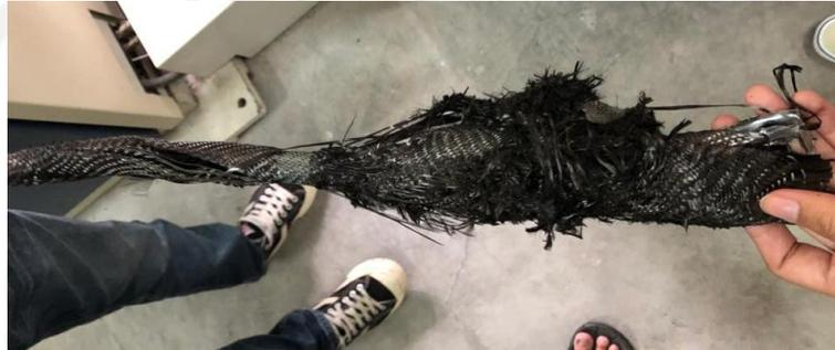
**Gambar 5.7 Carbon Fiber Trial I Setelah Diuji**
