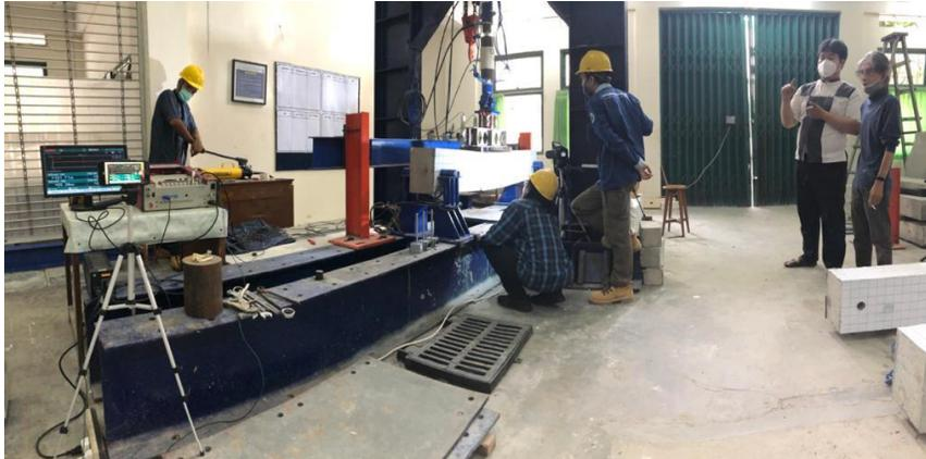
GAMBAR 39 PROSES PENGUJIAN KUAT LENTUR BETON
