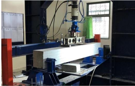
**Gambar 5.30 Setting Up Benda Uji Balok Beton**
