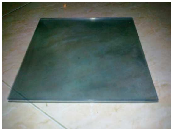
Gambar 3.5 Lembaran plastik PET ( polyethylene terephthalate )
