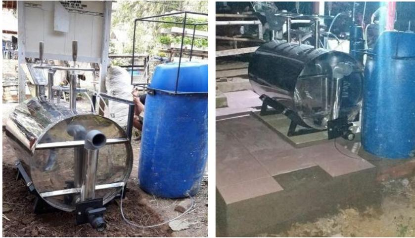
Gambar 5. digester portable plus desulfurizer
