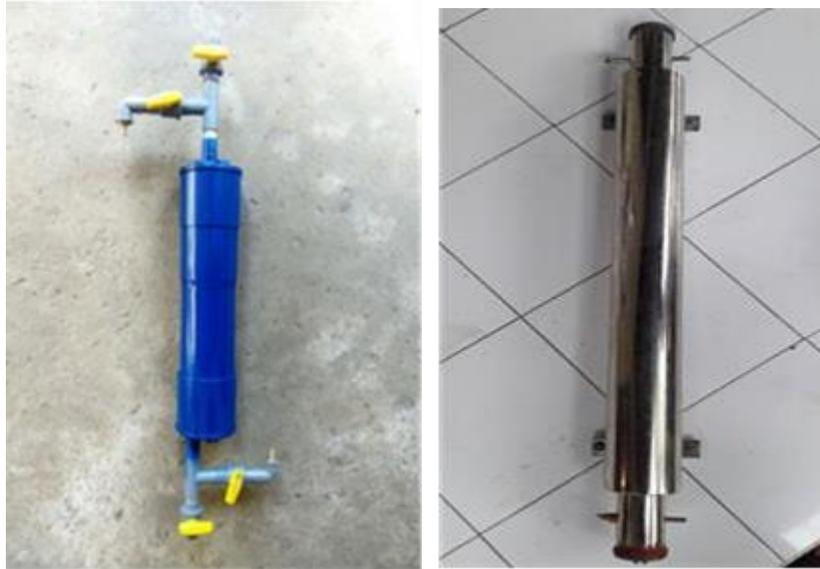
Gambar 1. Desulfurizer dan CO<sub>2</sub> remover
