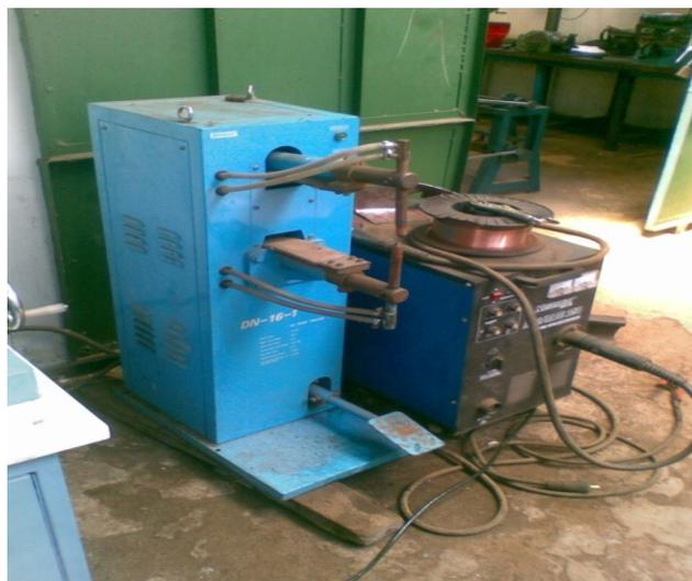
Gambar 3.4. Alat RSW (*Resistance Spot Welding*)
