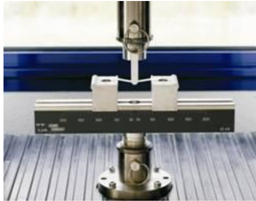
Gambar 2-5 Pengujian Bending strength metode tiga titik tumpu ( www.rtd.frwhy_post.php ) (7/05/2011)
