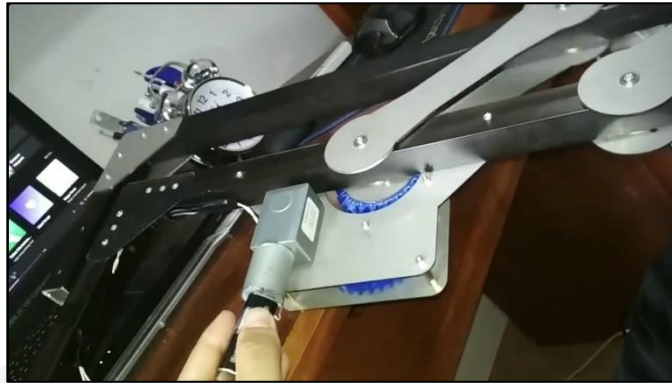
Gambar 4-24 Motor JGY-370 60 rpm
