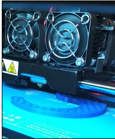
Gambar 3-41 Proses 3D Printing Hook
