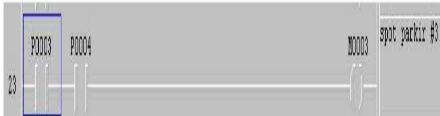
Gambar 2.9. Contoh fungsi Ladder Gerbang AND
