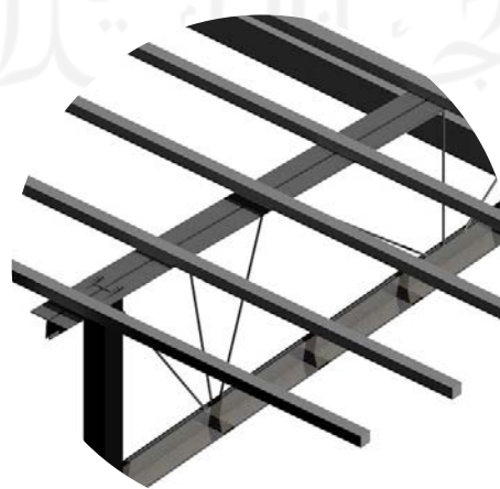
Frame Truss Roof Structutre
