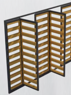
Secondary Skin Facade Module
