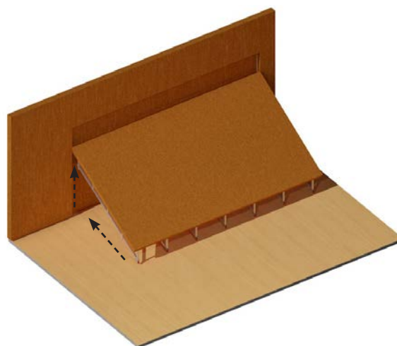
the process of retracting the stage
