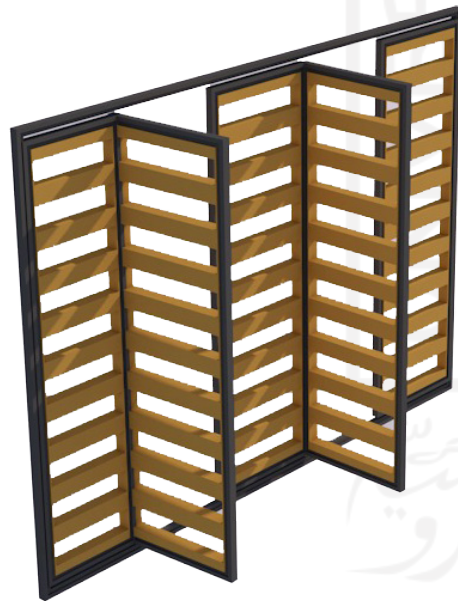
Secondary Skin Facade Module
