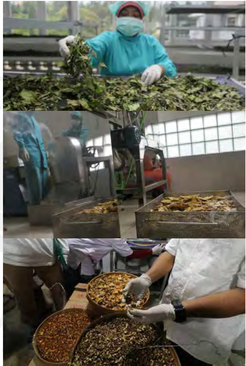
Figure 10. From Top: Ingredient Sorting, Drying, and The Result from Milling Process.
