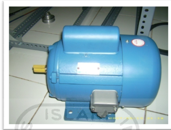
Gambar 3.8 Motor AC 1 phase \frac{3}{4} HP 1400rpm
