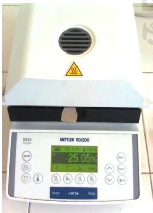
**Gambar 32. Alat uji kadar air**
