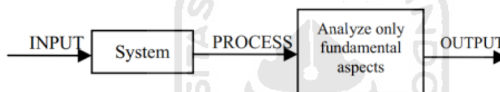
Gambar 2.3 Sistem Kerja Black Box Testing
