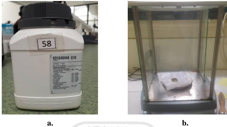
Gambar 3.5 Tahap Penimbangan (a. Asam Sitrat C_6H_8O_7 , b. Penimbangan Larutan Asam Sitrat C_6H_8O_7 )
