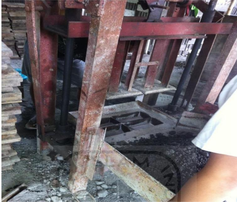
Gambar 1.8 Mesin Press *Paving Block*
