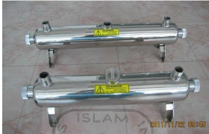
**Gambar 5. 7 Unit Ultraviolet**
