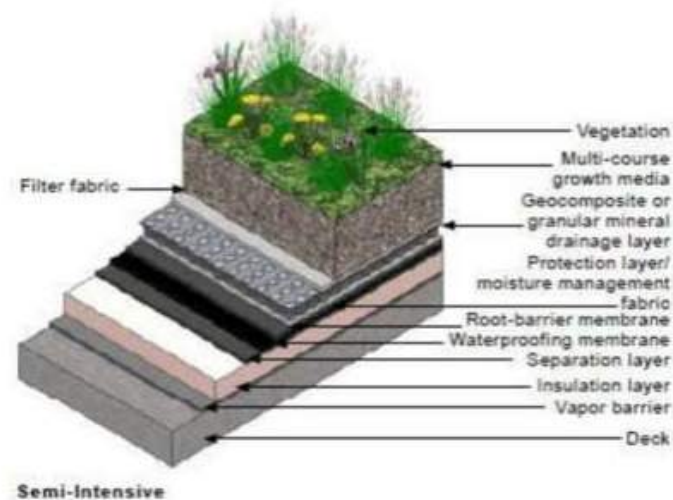
Gambar 2. 16 Semi Intensif Green Roof Sumber : Uptontraversecity, 2013
