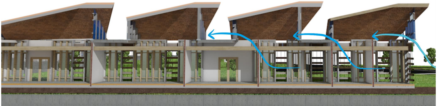
Figure 63 Mass 1 Natural Ventilation Design
