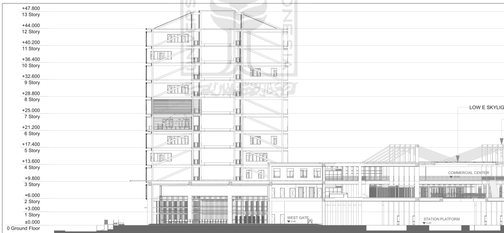
Figure 5.2.9: Mixed use building section B-B' Source: Author (2021)
