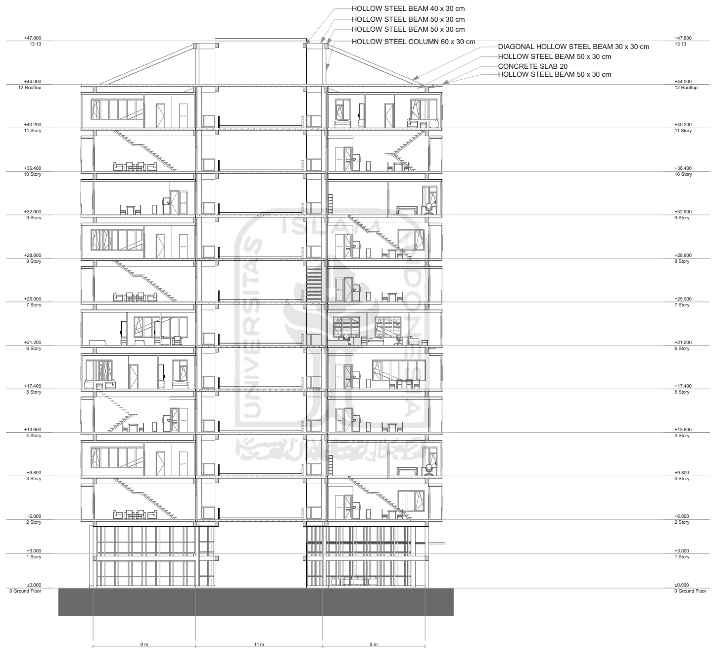
Figure 5.3.6: Apartment section A-A' Source: Author (2021)
