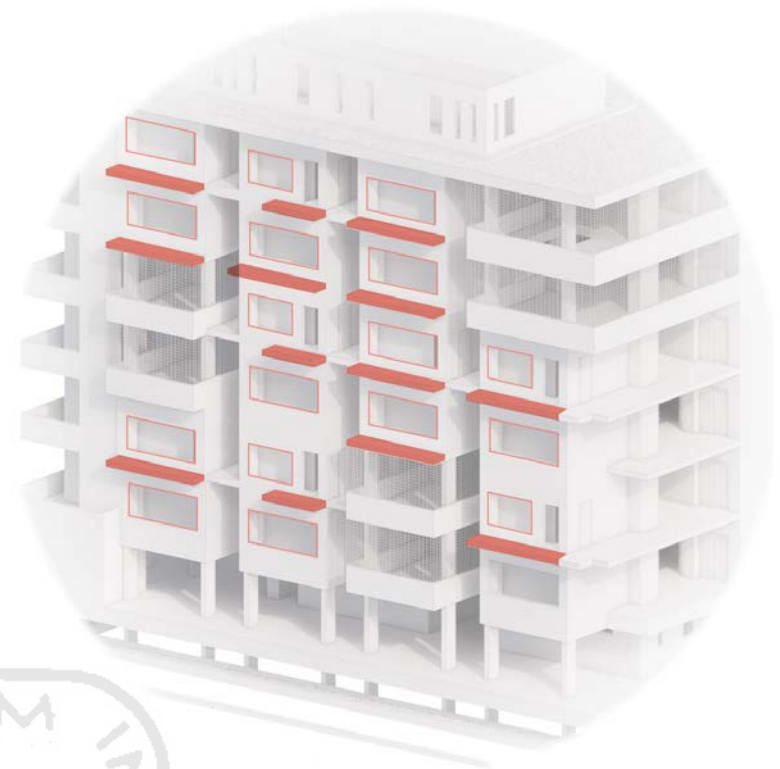
Hollow Space at Partition and Balcony Slab shown by the red color
