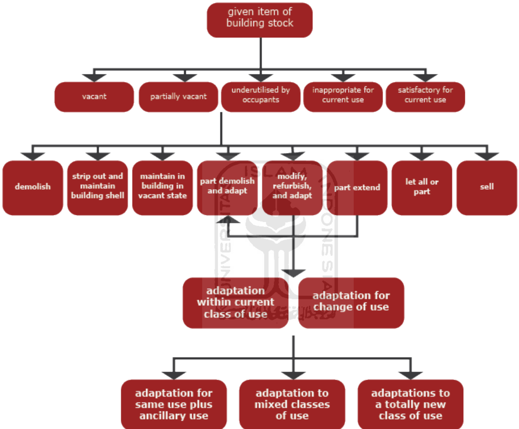
Figure 44: Basic options for adaptive reuse Source: Kincaid (2003)
