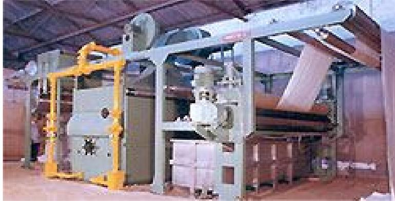
**Gambar 3.2** Mesin *singeing-desizing*
