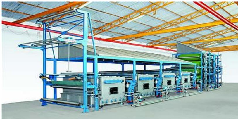
**Gambar 3.5** Mesin *washing-drying*
