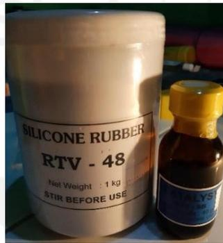
Gambar 2-11 *Silicone Rubber* RTV-48
