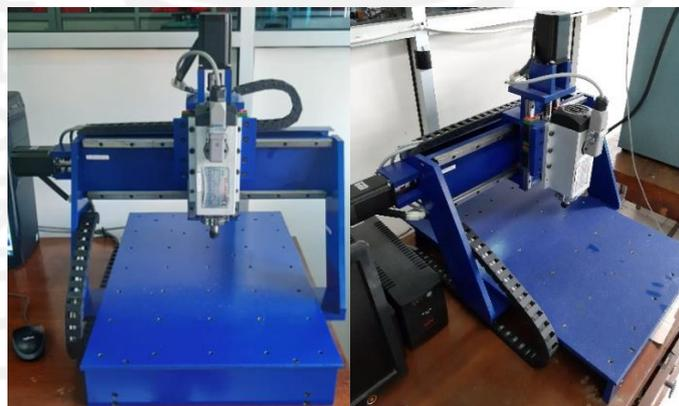
Gambar 2-7 Mesin CEDU CNC 3 Axis
