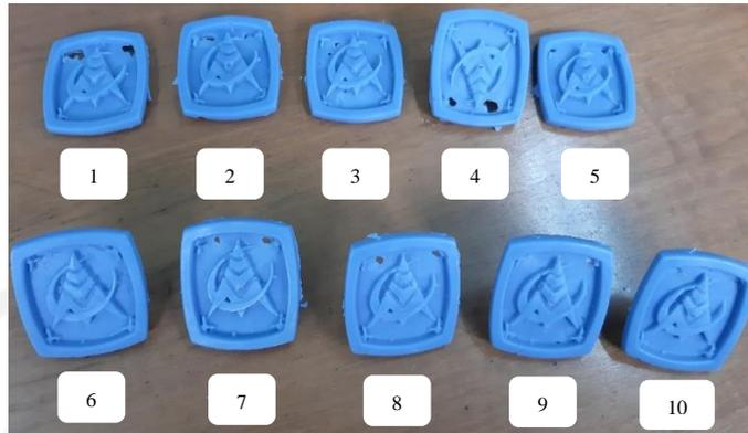
Gambar 4-15 Hasil Percobaan *Inject Wax* Silikon Model 3
