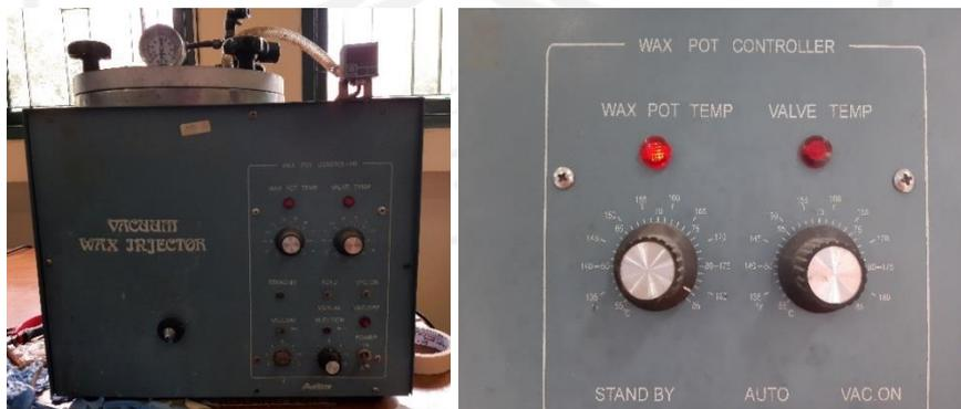
Gambar 2-12 *Vacuum Wax Injector*
