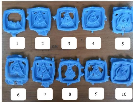
Gambar 4-10 Hasil Percobaan *Inject Wax* Silikon Model 1
