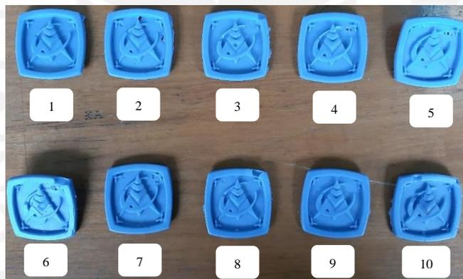
Gambar 4-17 Hasil Percobaan *Inject Wax* Silikon Model 4
