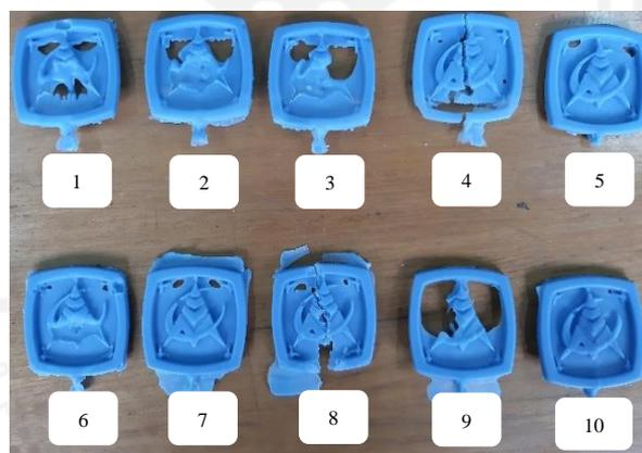
Gambar 4-12 Hasil Percobaan *Inject Wax* Silikon Model 2
