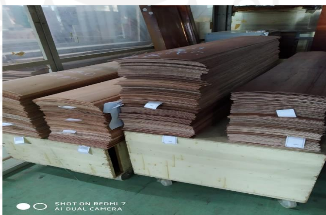
Gambar 5.4 Proses Pengeringan Veneer di Ruang Seasoning
