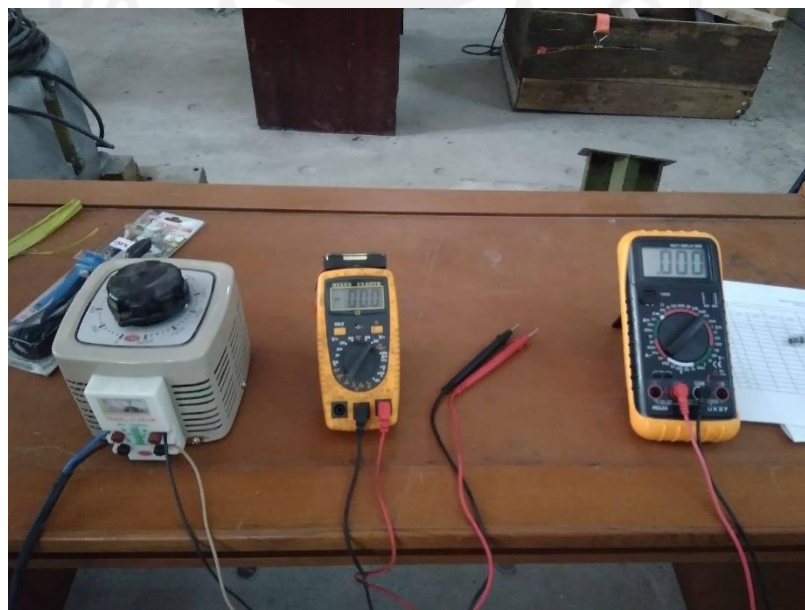
Gambar L-3. 18 AC Voltage Regulator, Multimeter
