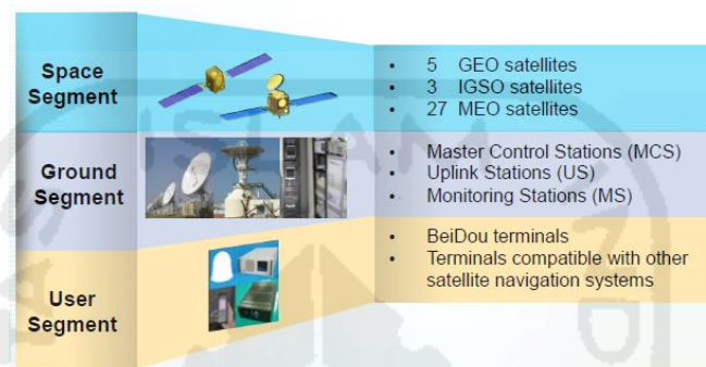
Gambar 2.4 Basic system of Beidou Navigation System
