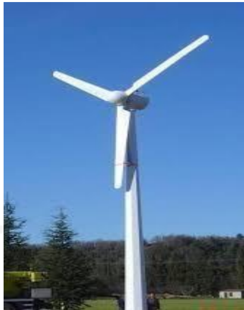
Gambar 2-2 Turbin sumbu Angin Sumbu Horizontal [10]
