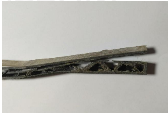
Gambar 4.7 Spesimen 5 Mengalami Gagal Core Failure
