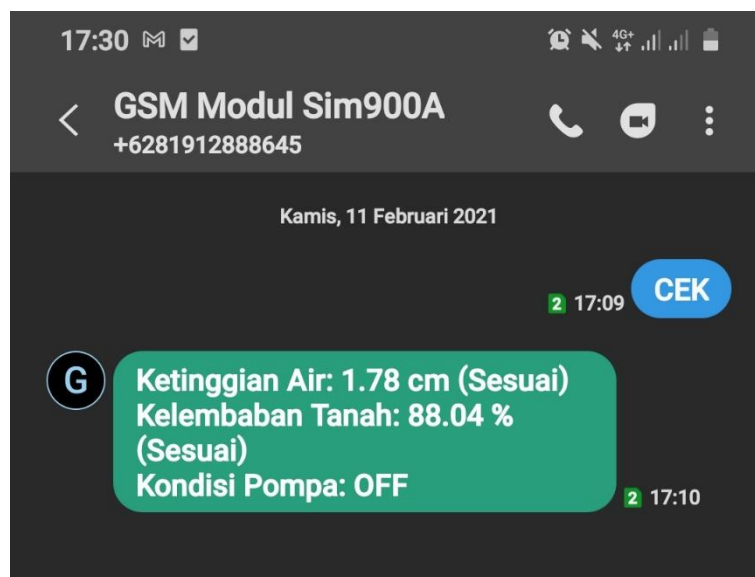
Gambar 4.13 Tampilan Monitoring Pompa Melalui SMS
