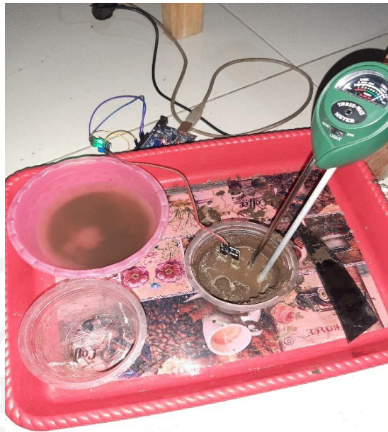
Gambar 4.2 Kalibrasi Sensor Kelembaban Tanah (YL-69)
