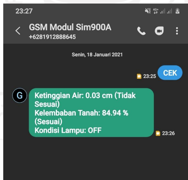
Gambar 4.11 Tampilan Monitoring Lampu Melalui SMS
