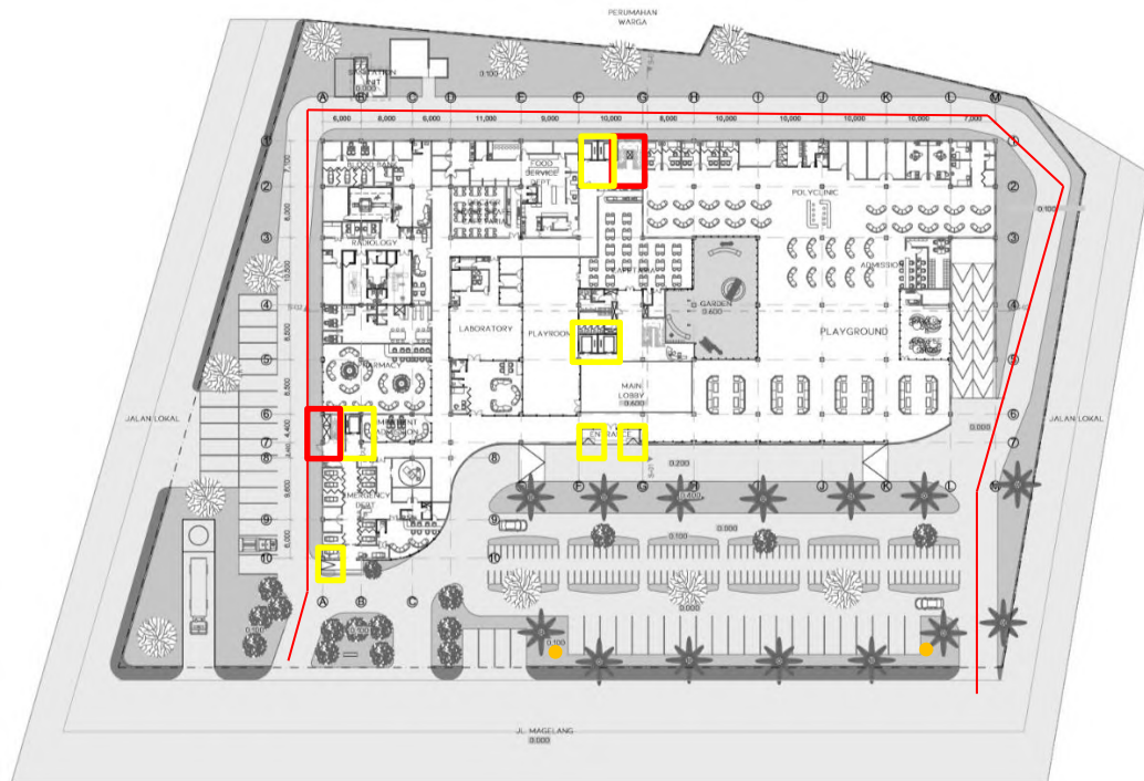
Gambar 175. Akses Difabel & Keselamatan Bangunan Ground Floor
