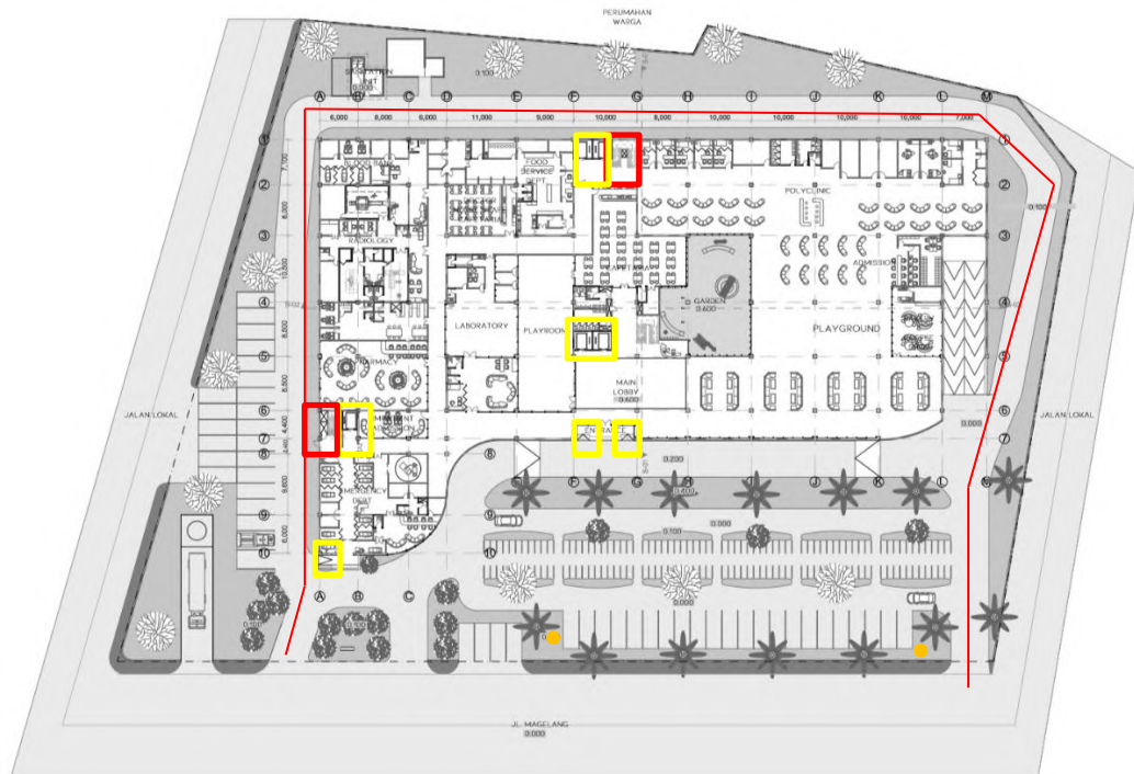
Gambar 108. Akses Difabel & Keselamatan Bangunan Ground Floor
