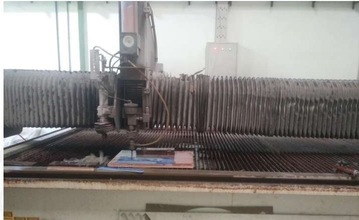
Gambar 4-10 Proses waterjet cutting
