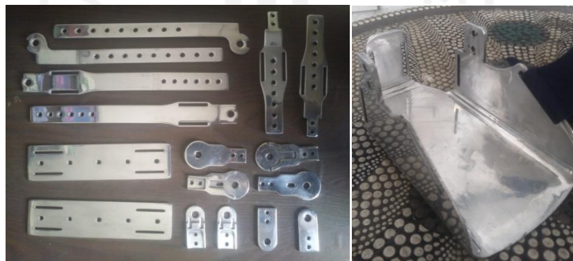
Gambar 4-15 Hasil finishing part
