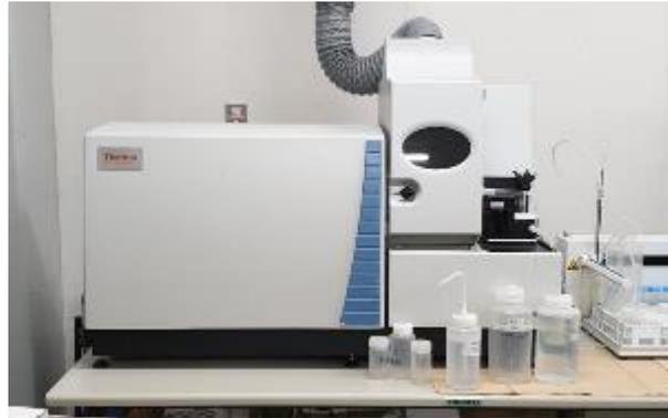
Gambar 7 Mesin ICP-MS X Series 2
