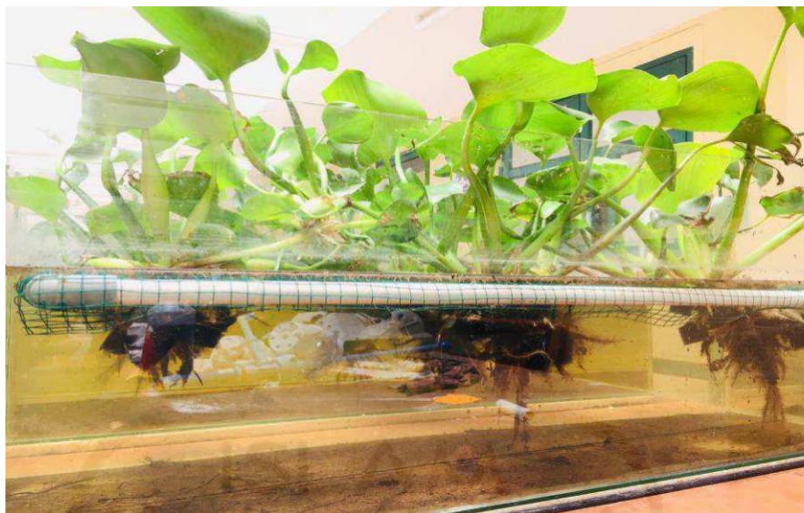
Gambar 24 Spons polyurethane di reaktor EFB+Spons
