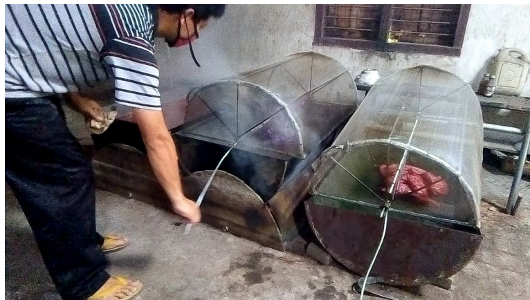
Gambar 4.23: Pengoperasian prototype alat pelorotan malam
