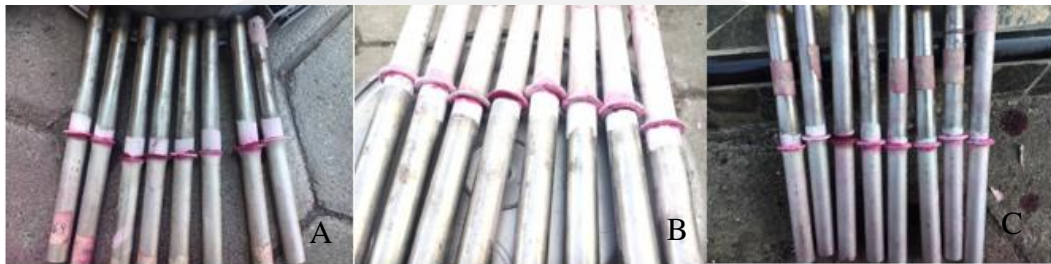
Gambar 4- 2 : Hasil Pengujian Dye Penetrant (A) 900 rpm, (B) 1170 rpm, (C) 1800 rpm
