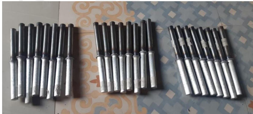
Gambar 4- 1 : Hasil Pegelasan A Variasi 900 rpm, B. Variasi 1170 rpm, C. Variasi 1800 rpm
