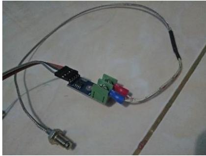
Gambar 3.6 Sensor suhu *thermocouple max 6675*.
