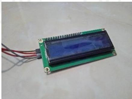
Gambar 3.8 LCD (*liquid crystal display*) I2C 16x2
