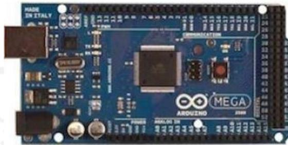
Gambar 2.8 Arduino mega 2560. [12]
