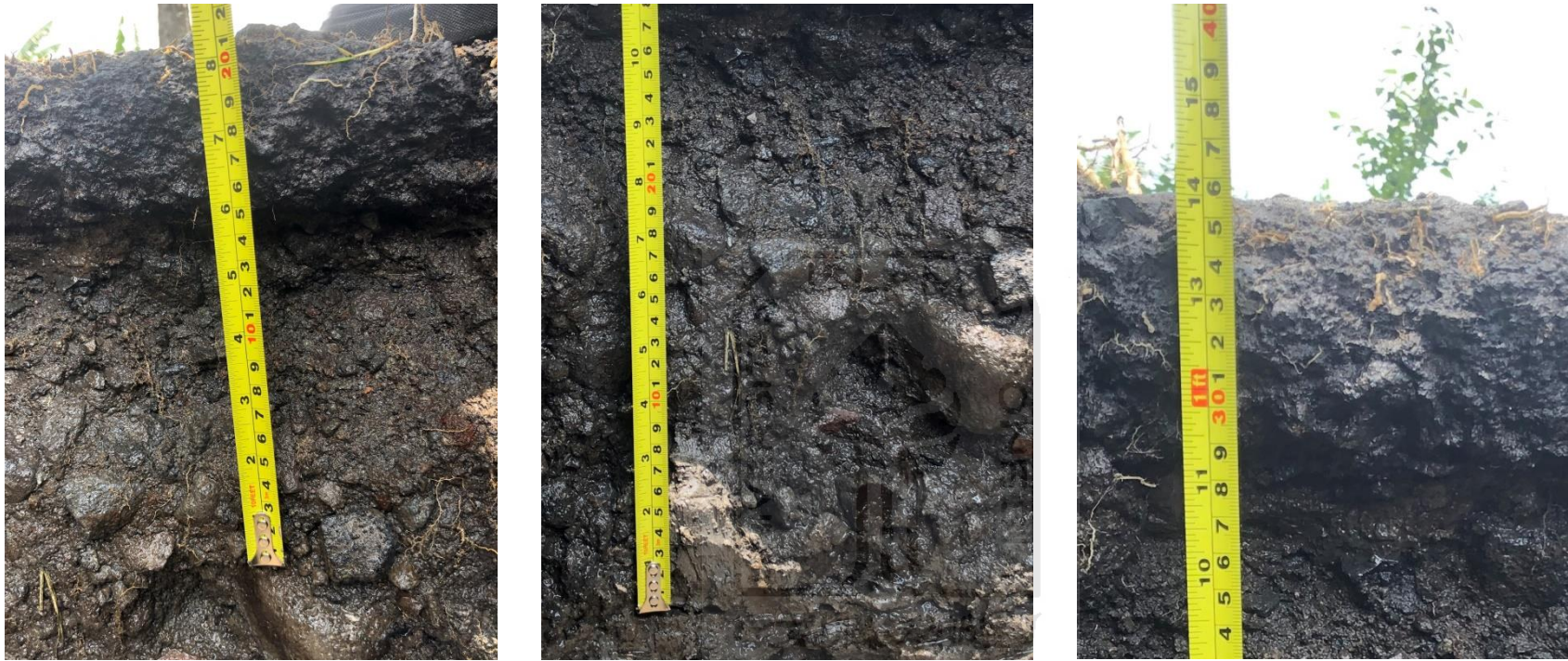
Gambar L – 5.5 Hasil Pengujian Test PITS STA 4+500
