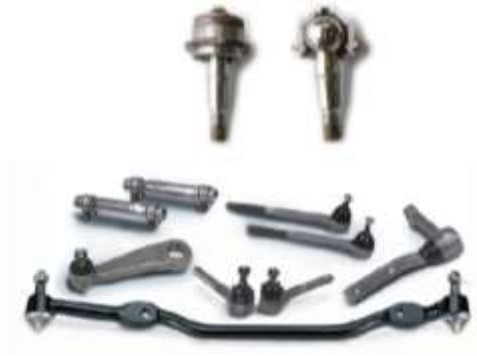
Gambar 2- 6 Macam - macam steering linkage
