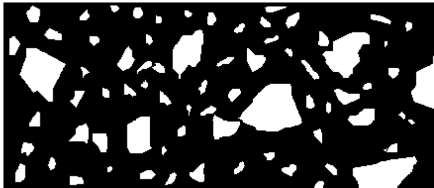
Gambar 3. 3 Campuran Split Mastic Asphalt (SMA)
