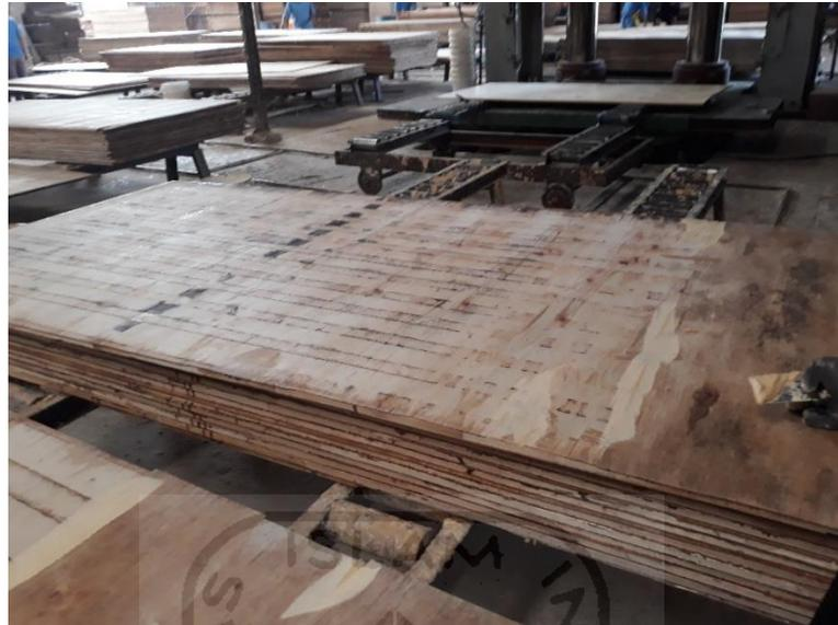
Gambar 4.18 Proses *Repair Kering*
