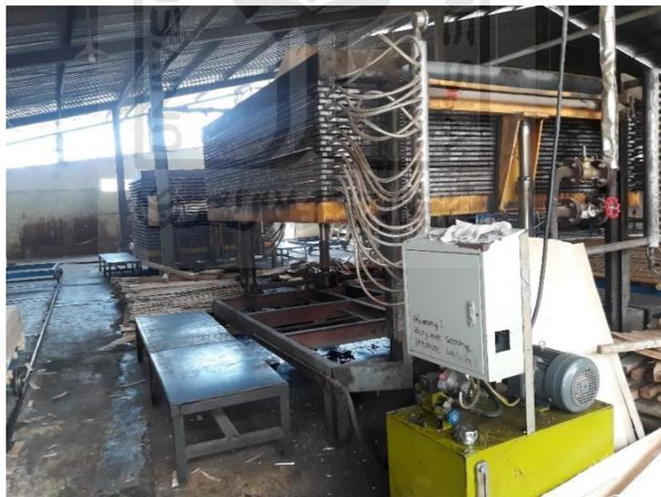
Gambar 4.11 Mesin *Press Dryer*
