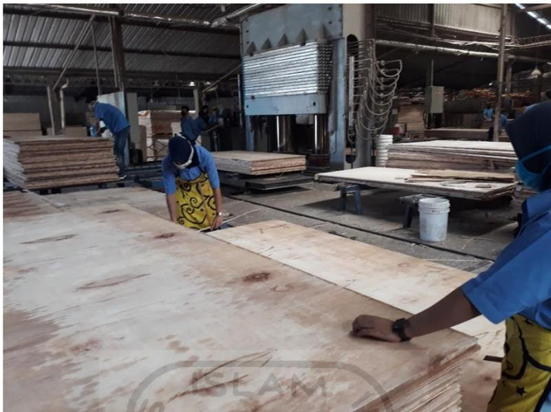
Gambar 4.16 Proses *Repair* Basah
