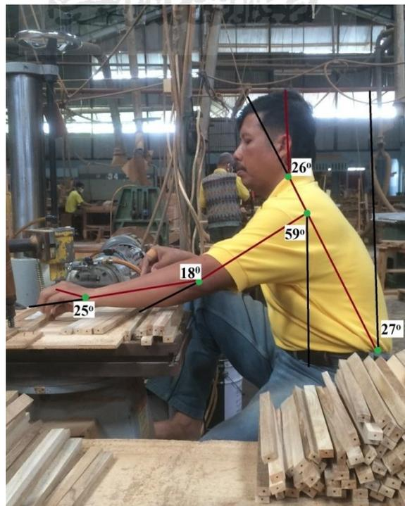
Gambar 4.3 Operator Mesin Horizontal Bor
