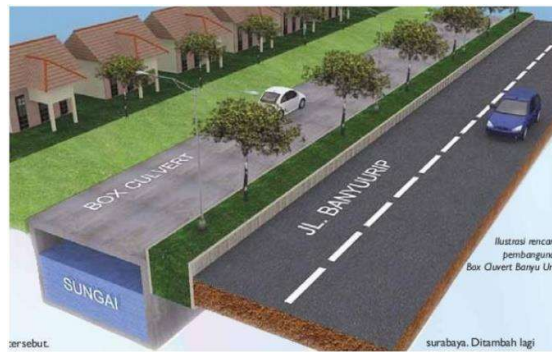
Gambar 2. 4 Gorong-gorong box culvert
