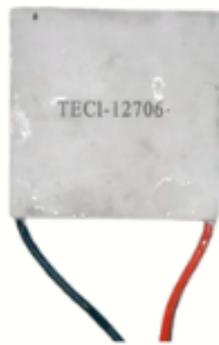
Gambar 3.2 Peltier seri TEC1-12706
