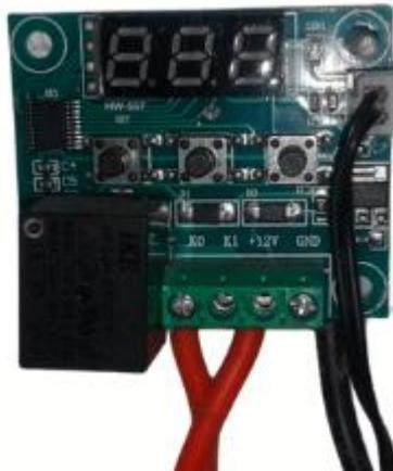
Gambar 3.5 *Thermostat Digital Professional W1209*
