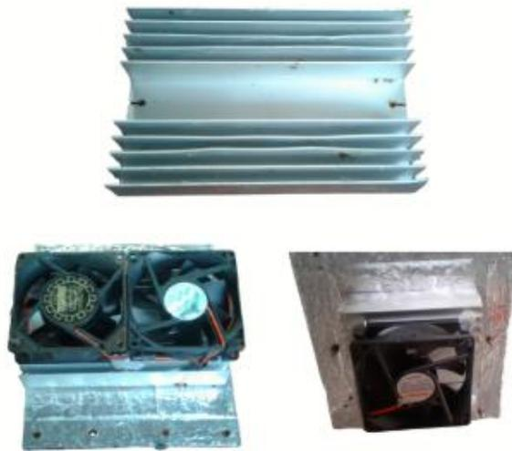
Gambar 3.4 *Heatsink Extruded* 10 sirip
